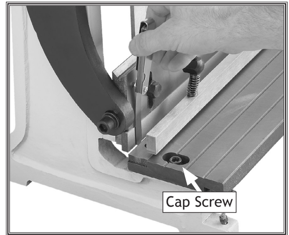
Figure 7. Checking shear alignment.
