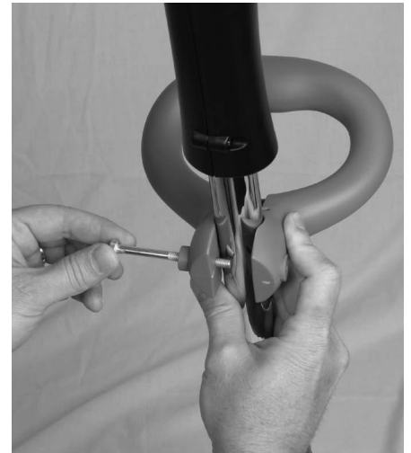
Figure 3-8: Inserting bolt into handle
