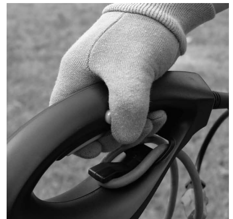
Figure 4-10: Squeezing trigger switch
