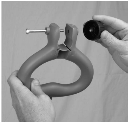
Figure 3-6: Removing knob and bolt from handle
