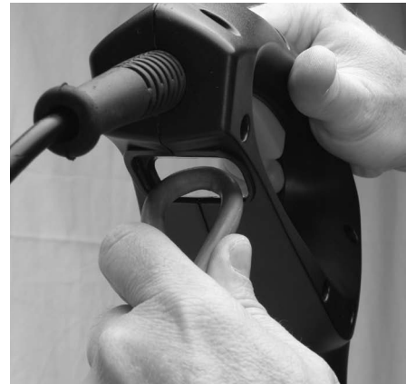
Figure 4-3: Inserting extension cord loop through bottom of handle
