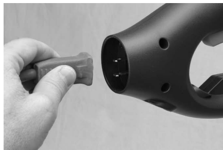
Figure 4-2: Plugging extension cord into inlet plug, Model RM112ST
