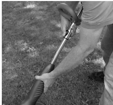
Figure 4-7: Adjusting shaft length
