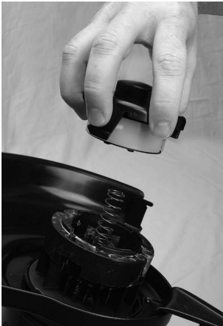
Figure 4-14: Removing spool cover and spool
