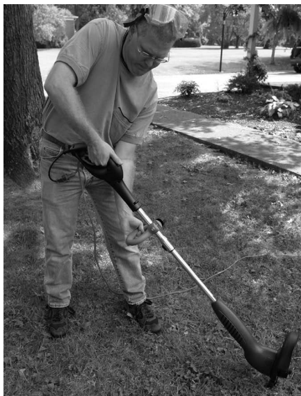
Figure 4-30: Rotating shaft and power head
