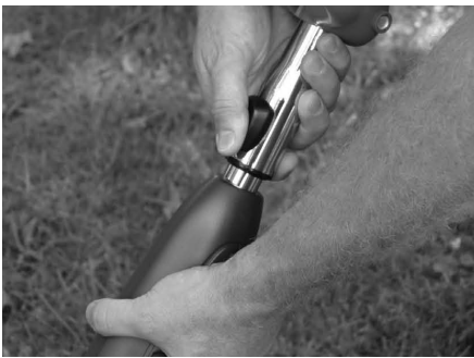
Figure 4-27: Sliding telescoping release button upward
