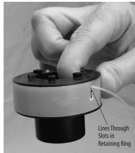
Figure 4-23: Positioning line in retaining ring slots
