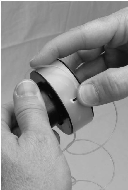
Figure 4-24: Winding line onto spool
