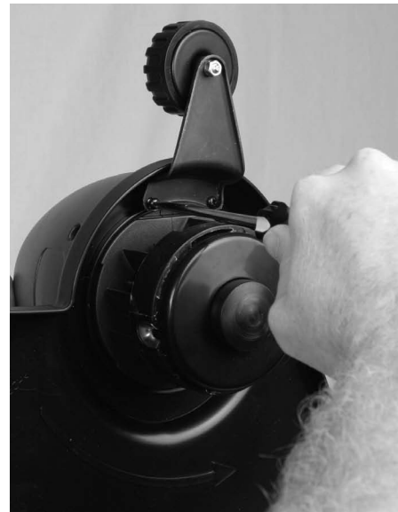
Figure 3-5: Attaching edging wheel
