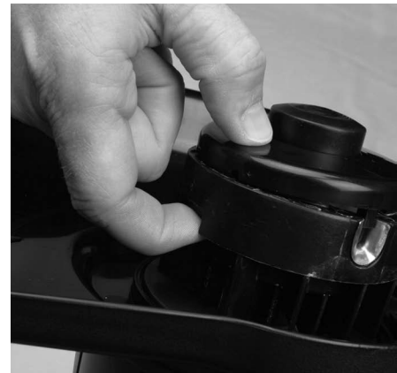
Figure 4-13: Unlocking spool cover
