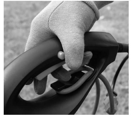
Figure 4-8: Holding trimmer/edger rear handle
