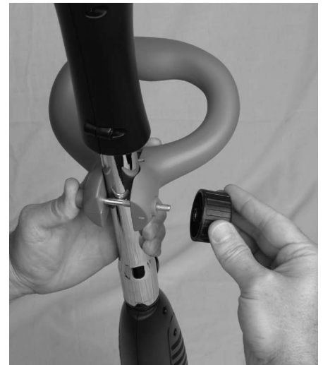
Figure 3-9: Screwing knob onto bolt
