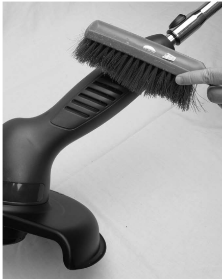
Figure 5-1: Cleaning trimmer/edger housing
