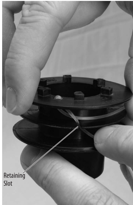
Figure 4-20: Arranging line into spool
