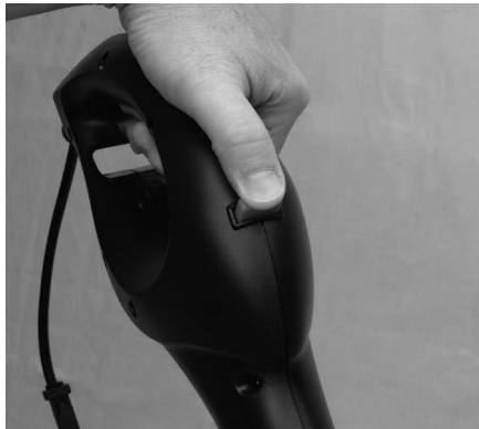
Figure 4-29: Pressing shaft rotation release button
