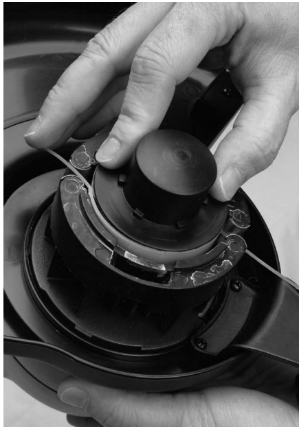
Figure 4-25: Replacing spool into spool housing
