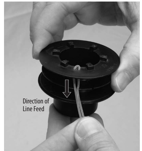
Figure 4-19: Pulling line tight
