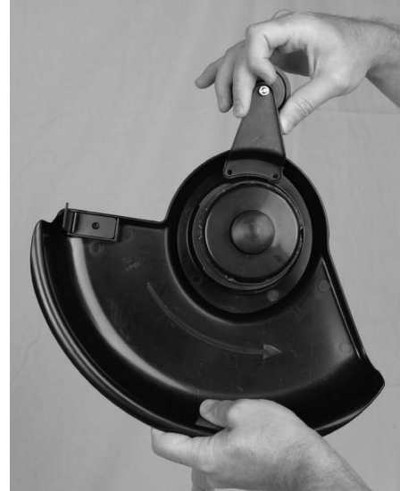
Figure 3-4: Placing edging wheel over screw holes
