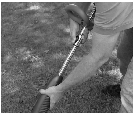
Figure 4-28: Adjusting shaft length
