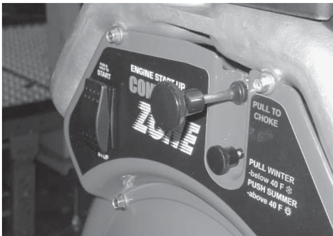
Figure 17 - Full Choke Position
