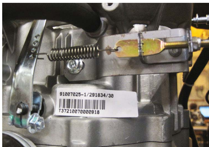
Figure 2.1 — Engine Governor Adjustment Single Cylinder Engines
