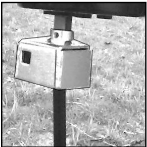
Adapter fits anchors and Soil Test Probe
