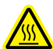
Burn Hazard / Hot Surface
