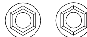
Engine to Engine Mount on Tank Part# 82281 M8-1.25 Ser Flange Nut Qty 4
