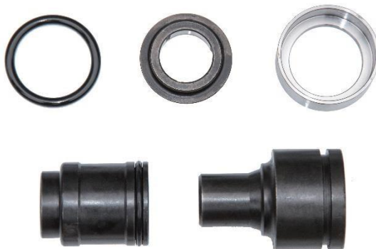
Figure 6: Damper assembly, hammer and anvil.
