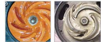
Tsurumi Impeller polished, not worn by abrasive material. Competitor Impeller is effectively worn out.
