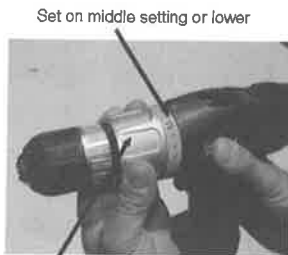
Turn to adjust clutch
